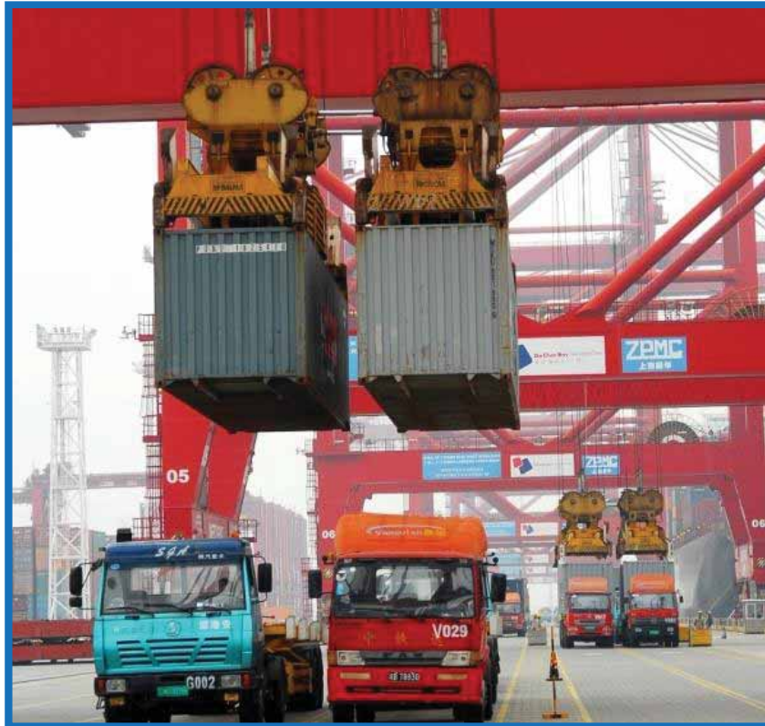
Figure 3.3-8 TANDEM LIFT STS CRANE Source: Da Chan Bay Terminal Website
