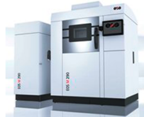
DMLS (Direct Metal Laser Sintering) Laser Sintered Metal Powder EOS M290 Build Volume: (9.8"x 9.8"x 12.8") Laser: 400-watt fibre laser Material: Stainless Steel Powder 17/4 PH
