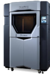
FDM (Fused Deposition Modeling) Stratasys Fortus 450 Build Volume: (16"x 14"x 16") Material: Polymer Filament Accuracy: \pm .005" (OR \pm .0015 in/in) Layer Thickness: (0.013 in to 0.005 in)
