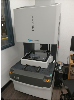
Optiv Classic (3D Probing & Optics) -Highly accurate measurement of small parts <15"
