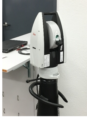
Leica AT960-LR (3D Probing & Laser Scanning) -Good for large volume measurements
